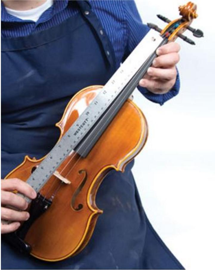
Usually the distance from the center of the bridge to the fret of the tailpiece (after length) is  $\frac{1}{6}$  that of the length of the strings measured from the center of the bridge to the fret of the fingerboard (effective string length).
