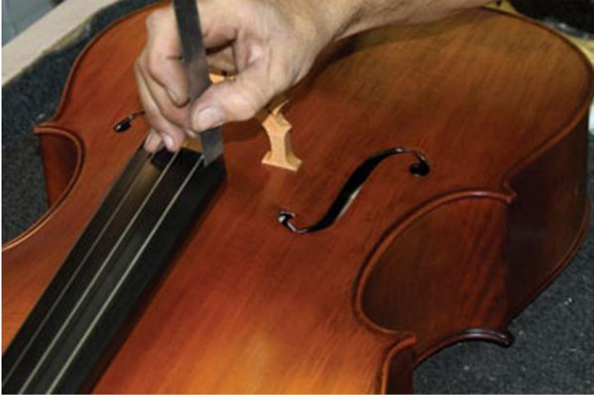
String heights are the distance between the strings and the top of the fingerboard measured at the end.
