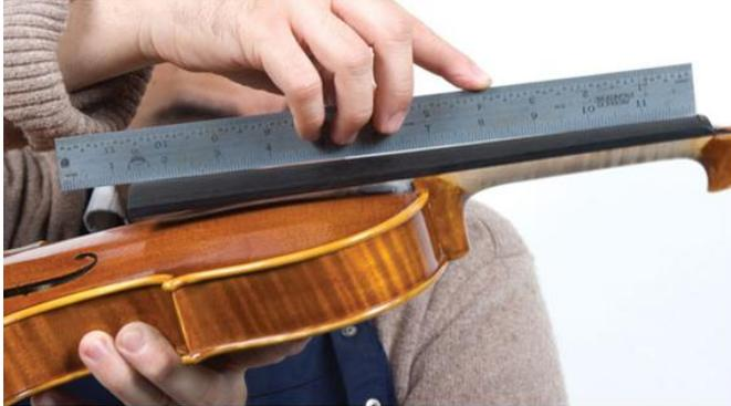
The highest points on the fingerboard are at each end. The amount of dip between these points is referred to as relief.
