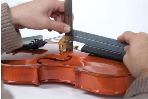
If the vertical angle or projection point is too low, the bridge and strings will be too low. As a result, the sound will be small and lack projection caused by too little tension on the bridge.
