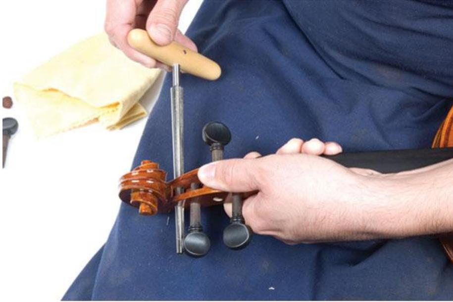
For a perfect contact, the taper of the peg reamer and the taper of the peg shaper must match perfectly.
