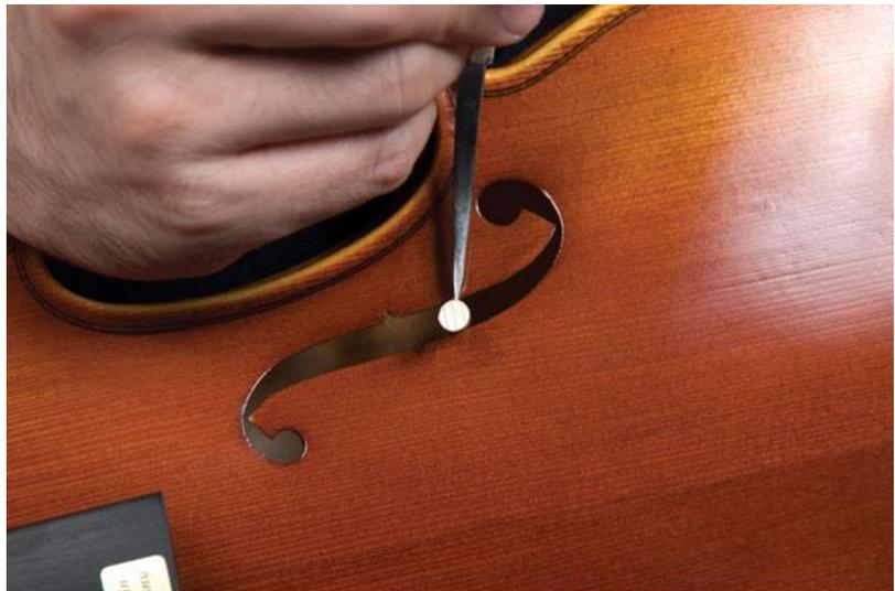
The soundpost grains must run perpendicular to the grains of the top plate.
