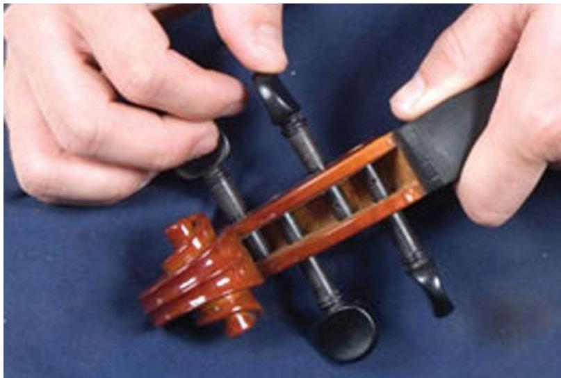
To check if pegs move evenly and easily, gently put pegs into peg holes (do not push hard). If they are well fitted, the pegs cannot be jiggled and will turn smoothly.
