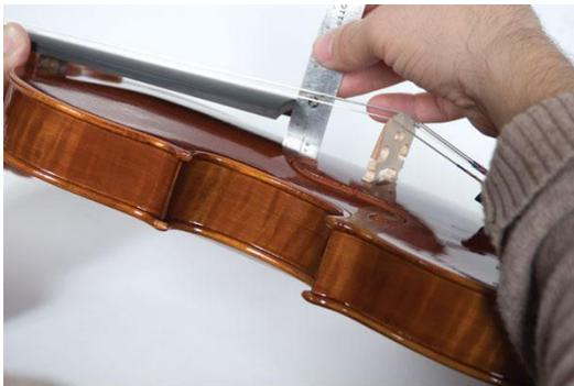
The vertical angle may also be measured at the highest point of the belly and at the end of the fingerboard. If the vertical angle is too high, the bridge and strings will be too high. Thus, the sound will be harsh and shrill caused by too much tension on the strings.
