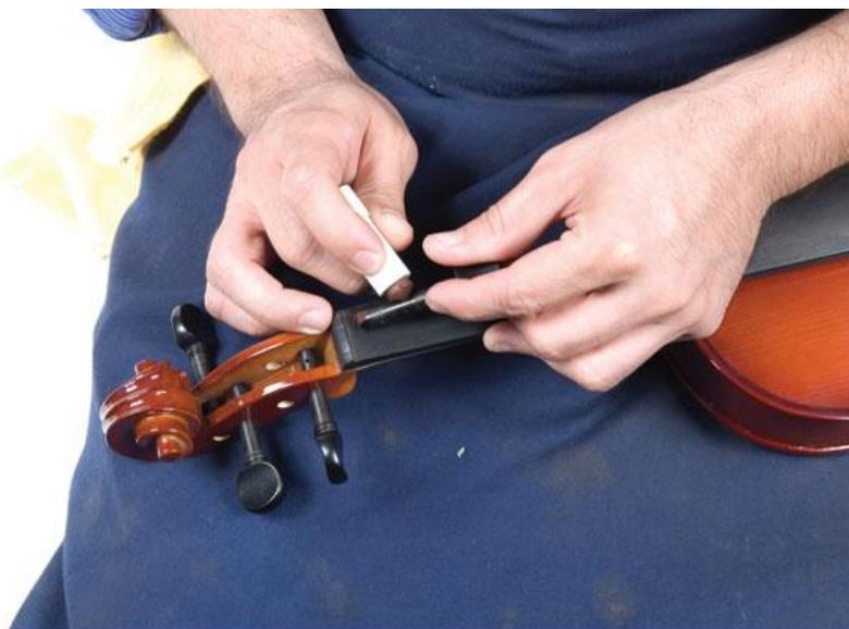
Pegs need to be properly lubricated from time to time for proper movement. We use Hill Peg Compound.
