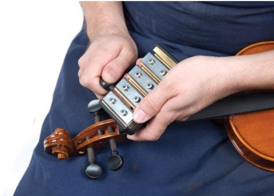
To achieve a perfect fit, the bulk of the wood removed must be taken from the peg, not the peg box. A peg shaper is used to remove this wood.
