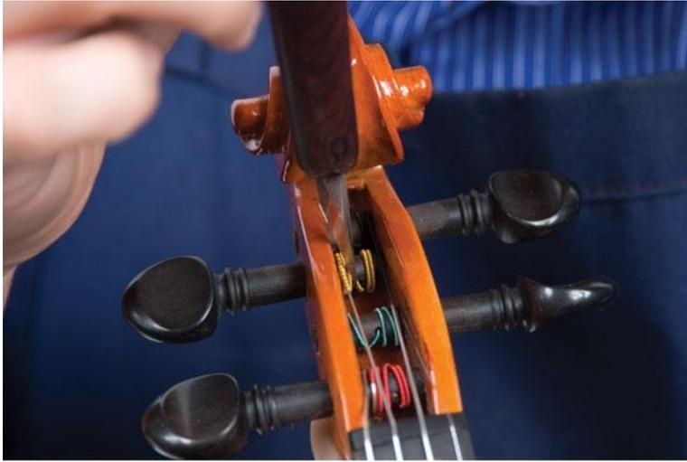
Both the placement of peg holes in the peg box and placement of string holes in the pegs are important for string performance and longevity.
